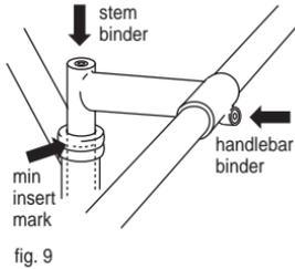
doesn't, get a piece of wood or a soft mallet and give the bolt a good whack to release the wedge. Adjust the stem position as desired, align stem with tire, and retighten the binder bolt tight enough so that you cannot twist the stem and handlebars out of alignment. **Under no circumstances should the stem be retightened with its "Minimum Insertion" or "Maximum extension" mark visible.**
